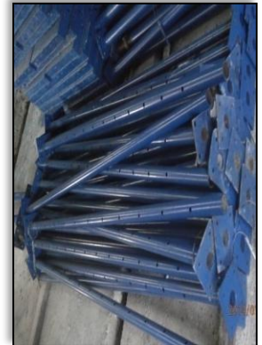
Shoring Jack 1.7m x 1.5m (3.10m extn.) 2.0m x 2.0m (3.8m extn.) 2.0m x 3.0m (4.8m extn.) 3.0m x 3.0m (5.6m extn.)
